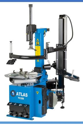
The TC320 is designed to ensure optimal efficiency with every tyre change, with a three point-assist arm for lifting and depressing of the bead, the equipment is designed to limit the potential damage to alloy wheels.
